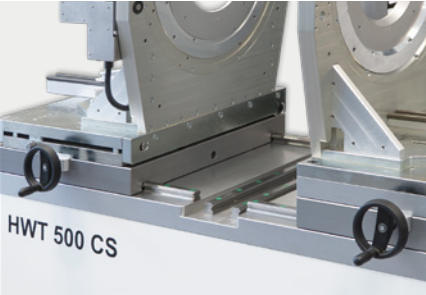
Horizontal adjustability of both carriages
