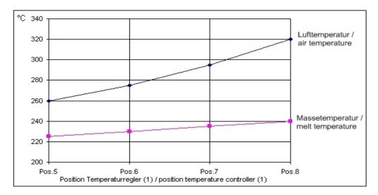
Check temperatures on the running extruder with an external thermometer after about 5 minutes.
