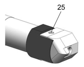
Care must be taken to ensure that the preheat nozzle provides intensive and uniform preheating (melting) of the base material over the entire joint width at as low a hot air temperature as possible. For larger weld seam widths, a wider preheat nozzle is available as an accessory.
