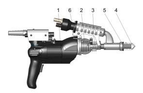
Type **MAK** is a hand extruder with integrated air supply (Autoair).
