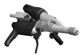
CAUTION Prior to prolonged interruptions of work (approx. 15-30min), set back temperature controller (1) by about 2 positions (risk of overheating of the melt in the melt chamber). Set temperature controller to welding temperature again approx. 5 minutes before resuming work.
