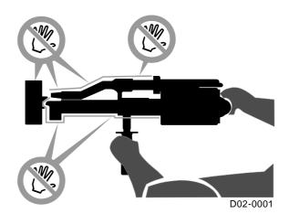
• Contact of combustible components with hot bare metal parts poses a risk of fire!
