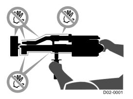
Always transport or store the hand extruder in such a way as to preclude any mechanical loads on the attachments.
