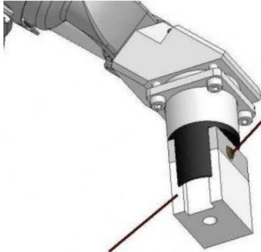
7. Welding shoes are turned in the desired direction and the quill screw is tightened.
