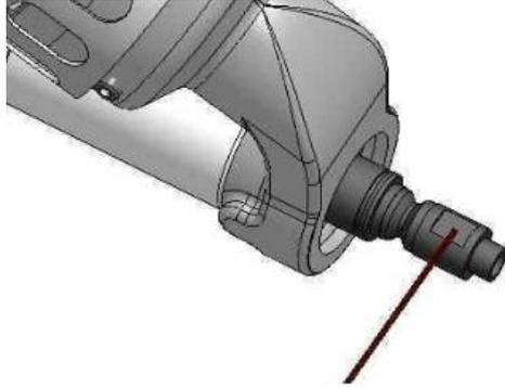
4. Nozzle (Ø 6 mm.) Screwed in (Left thread).
