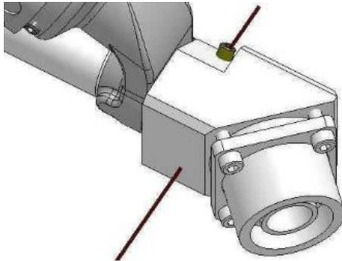
5. Angle head is mounted and screw is tightened.
