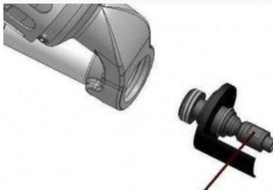
3. Nozzle (Ø 3 or Ø 4 mm.) with preheater nozzle unscrewed (Left thread).
