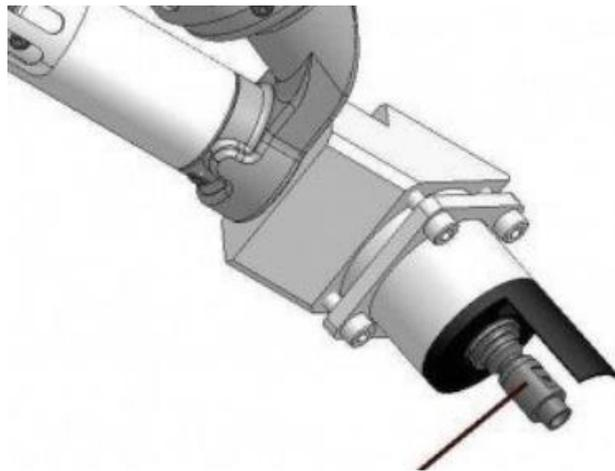
6. Nozzle (Ø 6 mm.) With preheater nozzle screwed in (Left thread).
